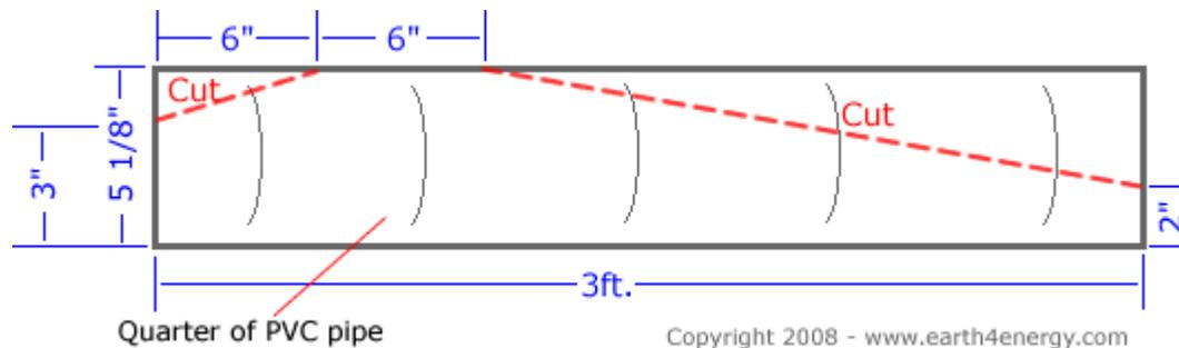
The wide part of the blade is what will help the windmill start spinning. The blade comes down to a narrow 2" tip, as this will allow the windmill to spin at high speeds.
