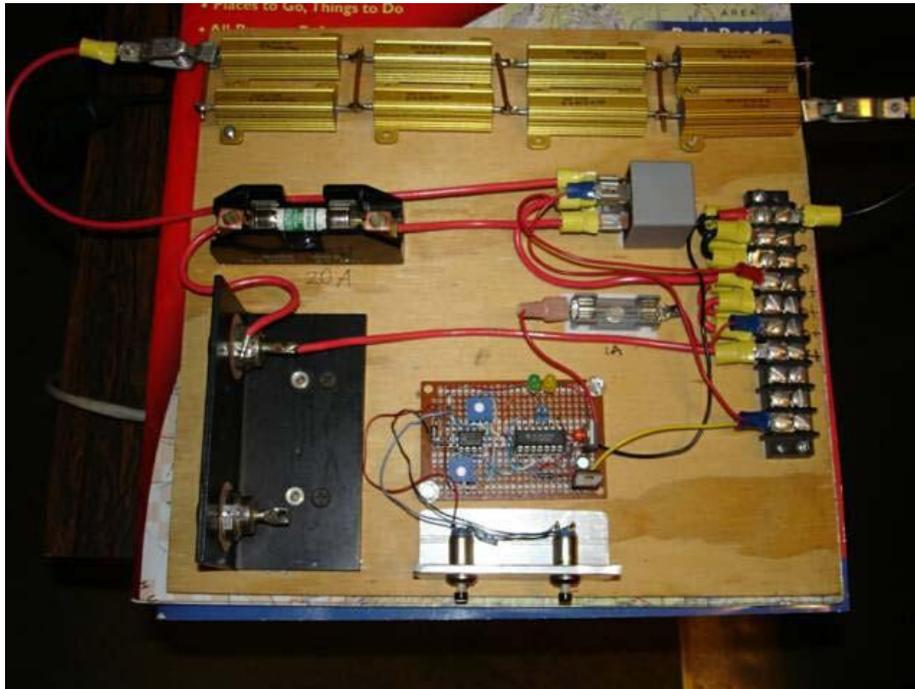
To determine when the wind turbine should stop dumping power into the battery, a charge controller must be attached. This necessity prevents the battery from over-charging, and wearing out too soon.
